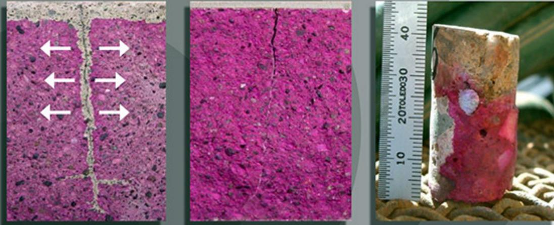
Carbonation of concrete is the result of a chemical reaction between carbon dioxide in the air and calcium hydroxide as well as hydrated calcium silicate in the concrete to form calcium carbonates. Over time carbonation reduces the pH, which ultimately leads to corrosion of concrete and loss of mechanical strength.
